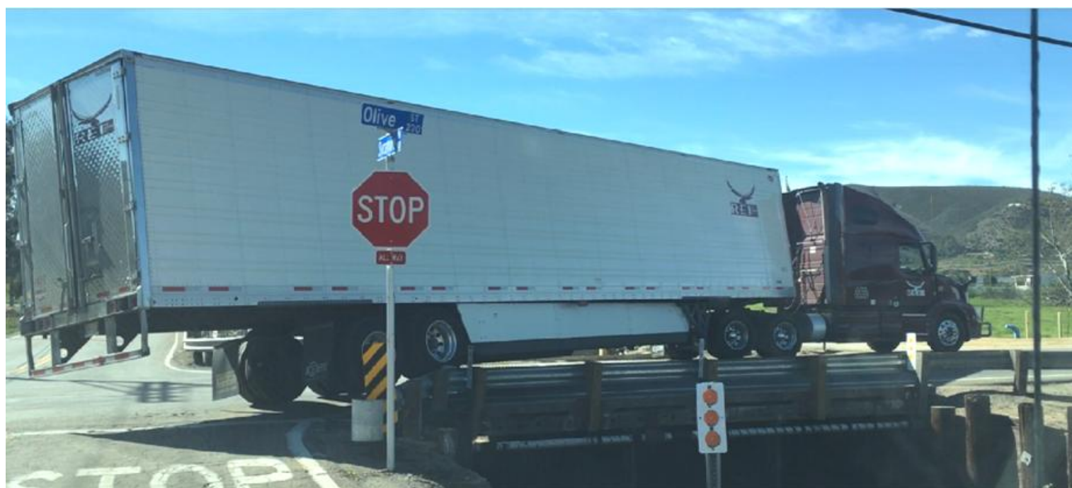
Semi-truck trailer attempting SB right turn from Sycamore Drive to Olive Street – wheels riding on top of guardrail
