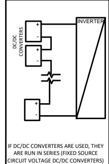
IF DC/DC CONVERTERS ARE USED, THEY ARE RUN IN SERIES (FIXED SOURCE CIRCUIT VOLTAGE DC/DC CONVERTERS)
