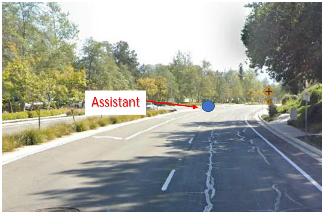
Measured Distance at the point where assistant can no longer be seen by the observer: at least 430 ft (East leg).
