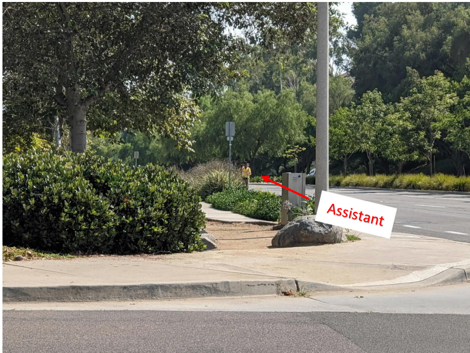
Measured Distance at the point where observer can no longer be seen by the assistant: 185 ft (East leg).
