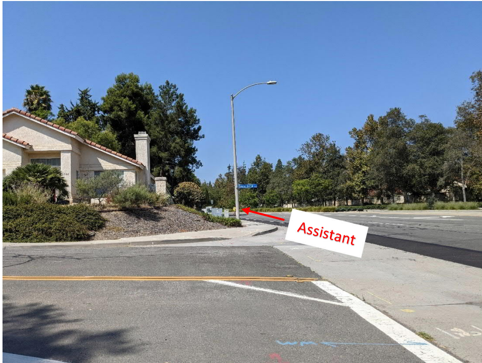
Measured Distance at the point where observer can no longer be seen by the assistant: 224 ft (West leg).
