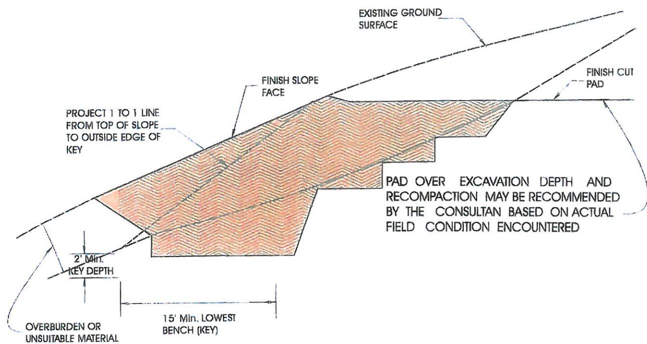
NOTE : SUBDRAIN DETAILS AND KEY WIDTH RECOMMENDATIONS TO BE PROVIDED BASED ON EXPOSED SURFACE CONDITIONS.
