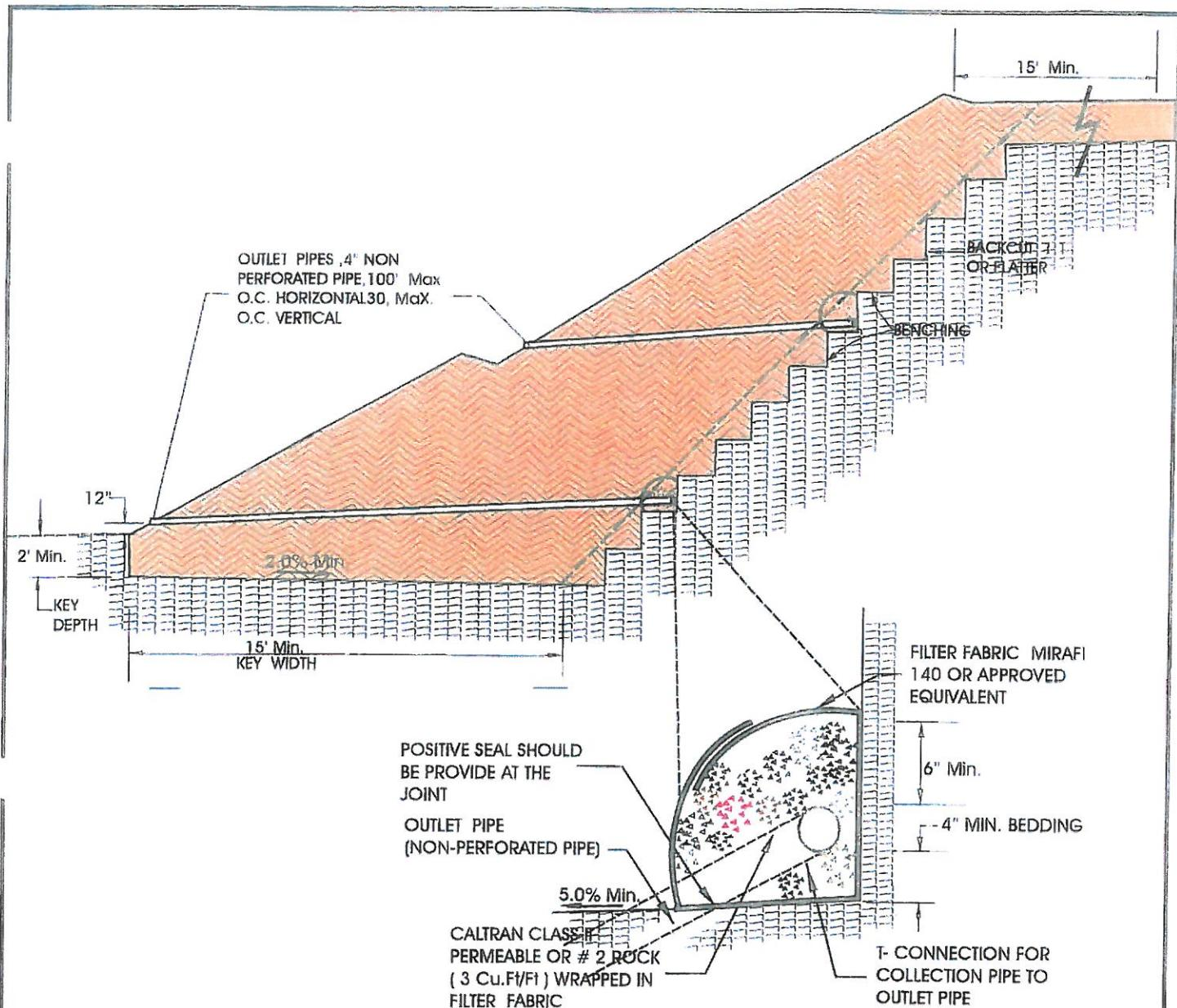
**SUBDRAIN INSTALLATION** - SUBDRAIN COLLECTOR PIPE SHALL BE INSTALLED WITH PERFORATIONS DOWN OR, UNLESS OTHERWISE DESIGNED BY THE GEOTECHNICAL CONSULTANT. OUTLET SHALL BE NON-PERFORATED PIPE. THE SUBDRAIN PIPE SHALL HAVE AT LEAST 8 PERFORATIONS UNIFORMLY SPACED PER FOOT. PERFORATION SHALL BE 1/4" TO 1/2" IF DRILLED HOLES ARE USED. ALL SUBDRAIN PIPES SHALL HAVE A GRADIENT AT LEAST 2% TOWARD THE OUTLET
